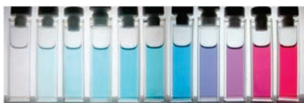
Figure 2. Play of colors in the reaction of TAA ( 5 \times 10^{-5} M) with \text{Cu}^{2+} . \text{Cu}^{2+} concentrations were 0, 0.2, 0.4, 0.6, 0.8, 1.0, 1.2, 1.4, 1.6, 1.8, and 2.0 equiv.
